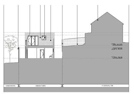
Figure 4: Central Section through the site showing relationship and gradient
